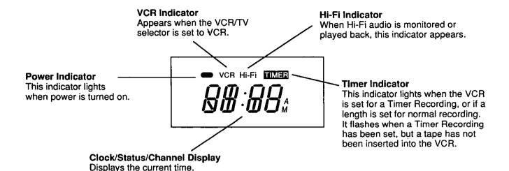
Briefly displays VCR status when function button is pressed. Also, briefly displays the channel number selected, "L" when
