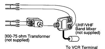
If your TV has both post and screw-type VHF terminals, using the post connection is recommended to minimize signal loss.
